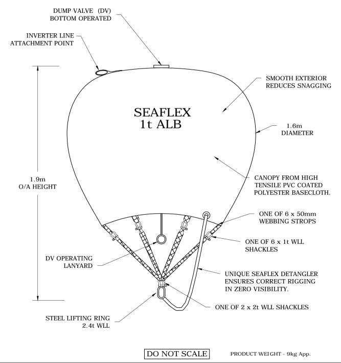
THE INTELLECTUAL CONTENT OF THIS DRAWING IS THE COPYRIGHT OF UNIQUE SEAFLEX Ltd. CONTENTS ARE ACCURATE AT TIME OF GOING TO PRESS, BUT MAY CHANGE WITHOUT NOTICE.
